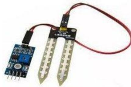
Fig.2. (Soil moisture sensor)
